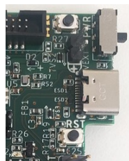
Fig.2.b– GAP9_EVK 3.0 onwards : USB-C + USB power on/off switch(Top right corner)
