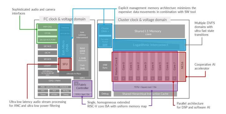
GAP9 is a unique combination of a powerful low power microcontroller, a programmable compute cluster with a hardware neural network accelerator and sample by sample audio filtering unit.
