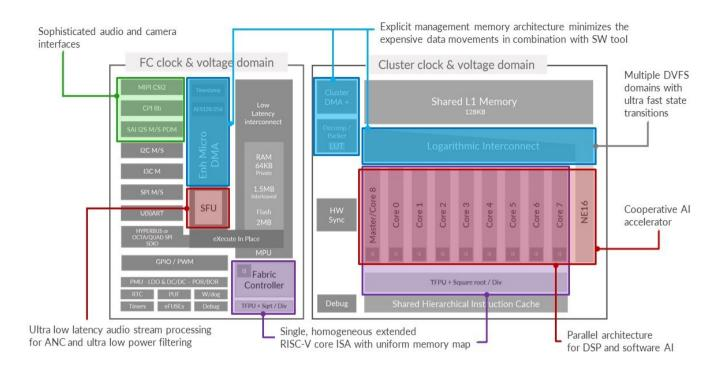
GAP9 is a unique combination of a powerful low power microcontroller, a programmable compute cluster with a hardware neural network accelerator and sample by sample audio filtering unit.
